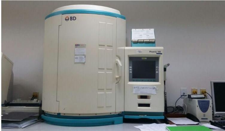
**Figure 4. BDPhoenix 100,automated system for the identification and susceptibility testing of clinically relevant bacteria** from Bicon Dickinson company, US.
