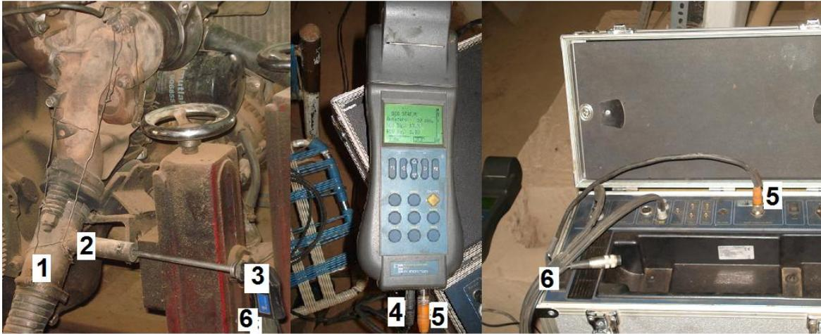
Fig (2): Flue gas analyzer. 1- Exhaust pipe. 2- Metal hole. 3- Steel tube and handle. 4- RCU power supply. 5- Communication cable. 6- Gas suction hose. 7- MCU power supply.
