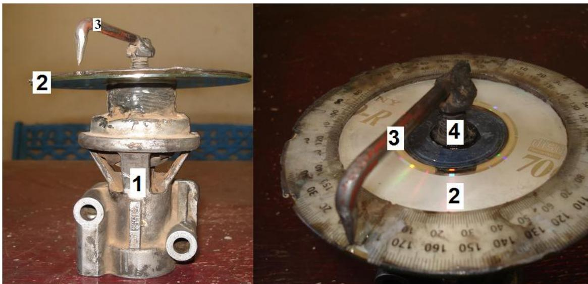
Fig (3): EGR valve. 1- EGR valve. 2 – 360deg. Protractor. 3 – Pointer. 4- Rotating bolt.
